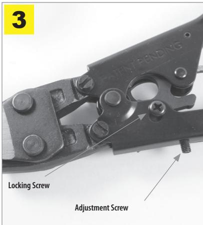
3. To adjust the jaw gap, turn the Pinch Tool on its side and locate the locking screw positioned on the handle. Use a standard screwdriver to loosen the locking screw. Locate the adjustment screw. Turn the adjustment screw right or left as needed to change the size of the jaw gap. When adjustment is complete, tighten the locking screw.
