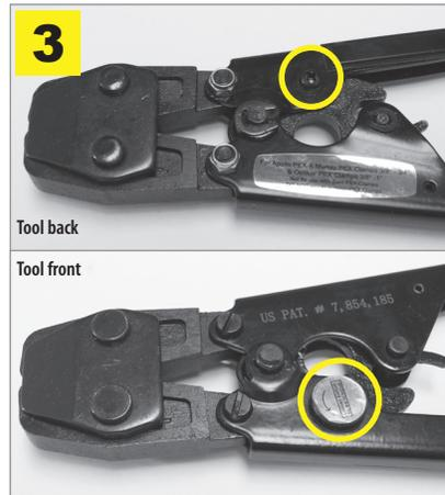
3. To adjust the jaw gap, turn the Pinch Tool on its back and locate the locking screw. Use a standard screwdriver to loosen the locking screw. Turn the tool over and locate the adjustment dial. Turn the adjustment dial right or left as needed to change the size of the jaw gap. When adjustment is complete, tighten the locking screw.
